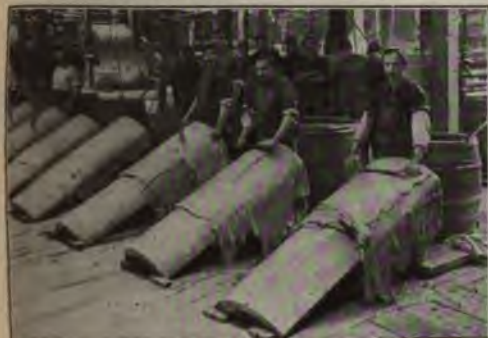
Four steps in the manufacture of leather. The first view shows the process of removing the hair from the hides and trimming the sinews, flesh, and other useless parts from them.
